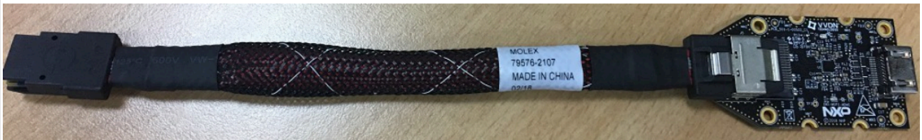
Figure 20. i.MX Mini SAS cable with DSI-to-HDMI adapter IMX-MIPI-HDMI
