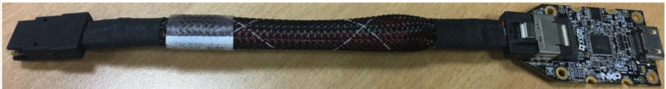
Figure 10. i.MX mini SAS cable with LVDS-to-HDMI adapter
