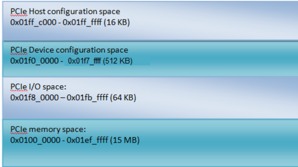
Figure 14. Memory Layout (i.MX 6Quad/6DualLite/6Solo)
