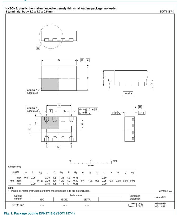
DFN1712-8: plastic thermal enhanced extremely thin small outline package; no leads; 8 terminals
