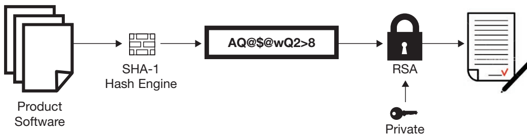
RSA/SHA-1 signature generation applied on Manufacturer code
