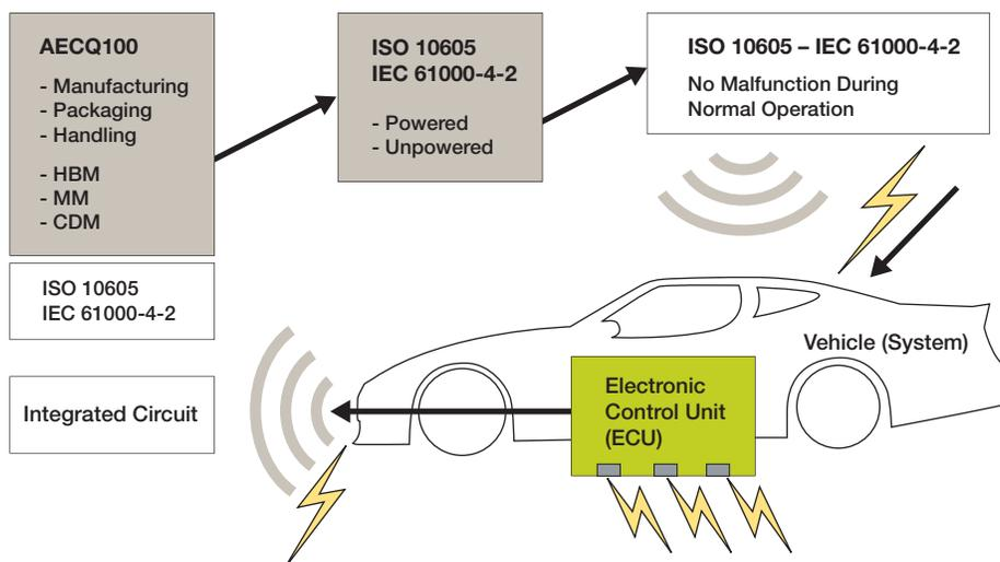
The CAN H and CAN L pins are designed to be strongly immune against system level stress directly applied at the pin level with and without external protections. To achieve such high performance (up to 25 kV), the SEED [7] approach (System Efficient ESD Design promotes an IC/OEM co-design methodology of on-board and on-chip ESD protections to achieve system level ESD) has been used. As an example the ESD performance of Freescale's CAN high speed physical layer is summarized in the table below.
