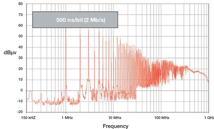
In order to remain inside the EMC level targeted by car makers, optimization of the CAN driver is required, to allow operation in CAN flexible data at 2 MB/s in a first step, and at high baud rate in the future.
