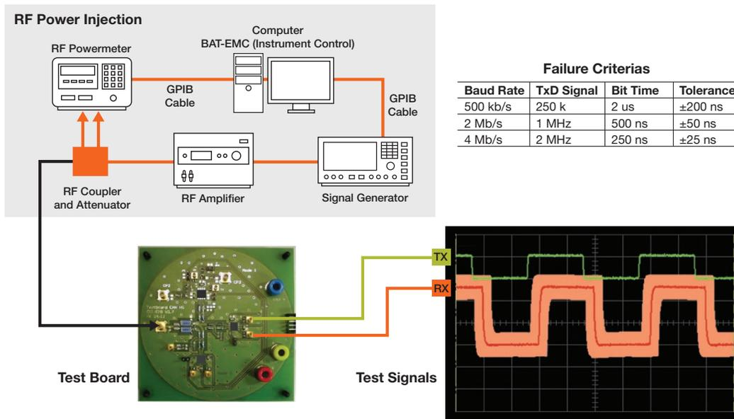
At the physical layer side, it results in a complete design for EMC flow that includes accurate design and layout guide lines, an extensive simulation on block level and top cell level, and models that include process and temperature variations inside EMC simulation runs, to ensure a certain margin versus the specification. As a consequence, these design improvements lead to a CAN signal integrity that supports signal injection up to 39 dBm.
