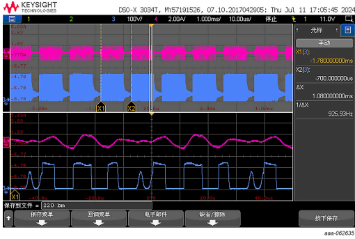
Figure 12. Operation in Burst mode (A) Operation in Burst mode at 220 VDC mains CH3: V_{HB} (100 V/div) CH4: I_{CR} (2 A/div) Time: 1 ms/div; 10 us/div
