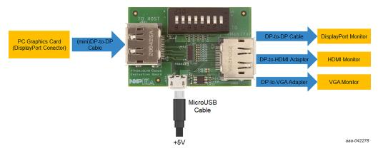
The PTN3816EVM evaluation board should be powered with a 5 V power supply using a MicroUSB cable (J404). DisplayPort connector on the left side of the board (J401, marked as "TO HOST") should be connected to a PC's graphics card through a DisplayPort Cable. DisplayPort connector on the right side of the board (J402, marked as "TO Monitor") can connect to one of the following for evaluation purposes:
