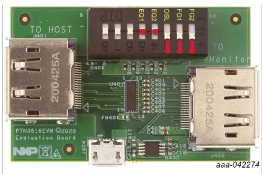
Figure 4. PTN3816EVM evaluation board control switches
