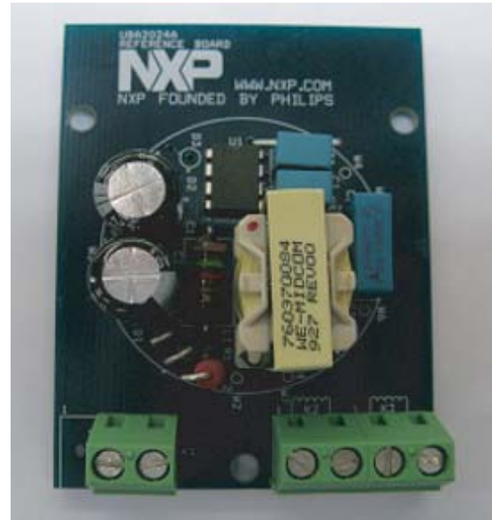
Fig 4. UBA2024P 120 V (AC) mains demo board
