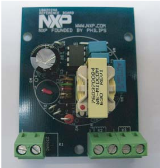
Fig 3. UBA2024P 230 V (AC) mains demo board
