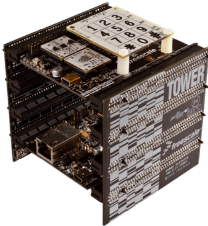
Figure 2 - Tower System with TWR-SENSOR-PAK
