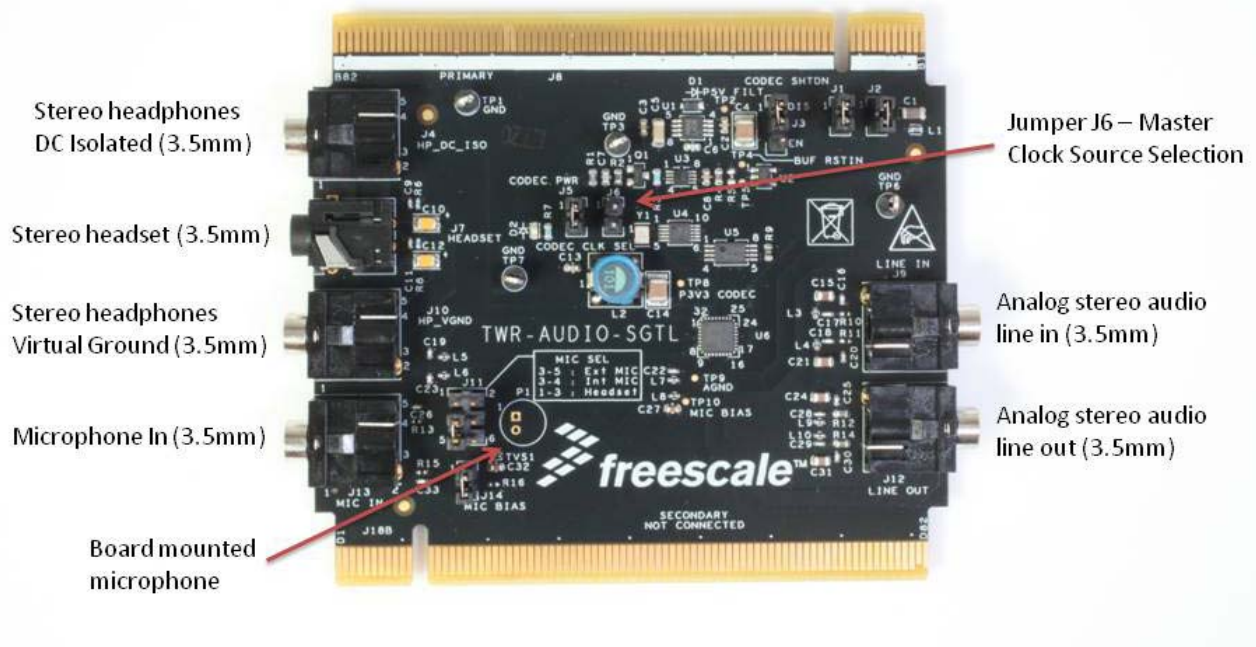
Figure 2. Callouts on top side of the TWR-AUDIO-SGTL
