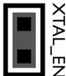
Figure 6-21: External Crystal Circuitry Enable (CT4)
