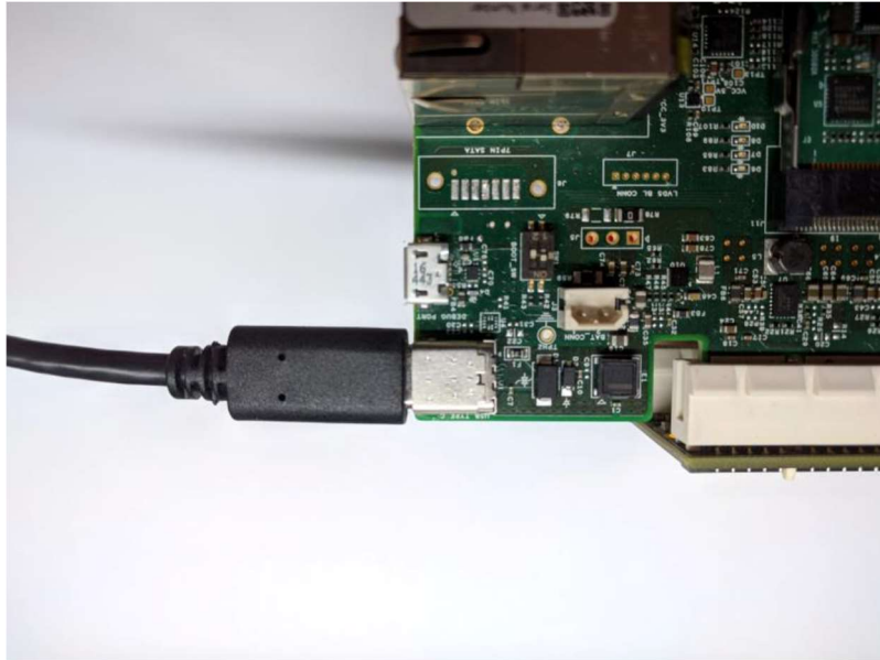
Figure 5. USB Type-C connected to the TWR-POS- i.MX6UL board
