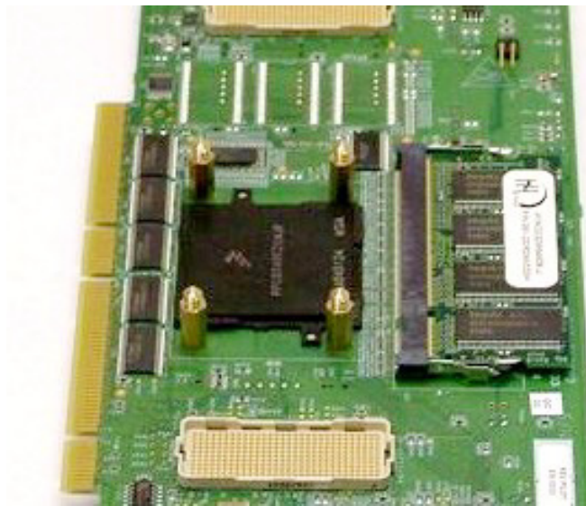
Figure 7-14 Heat sink removed
