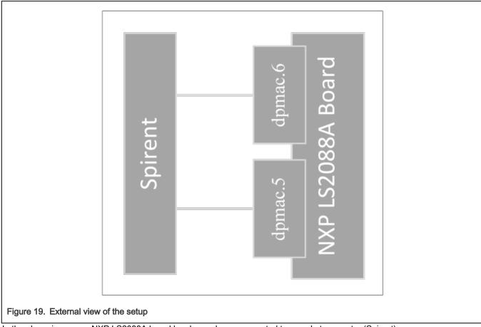
In the above image, an NXP LS2088A board has been shown connected to a packet generator (Spirent).
