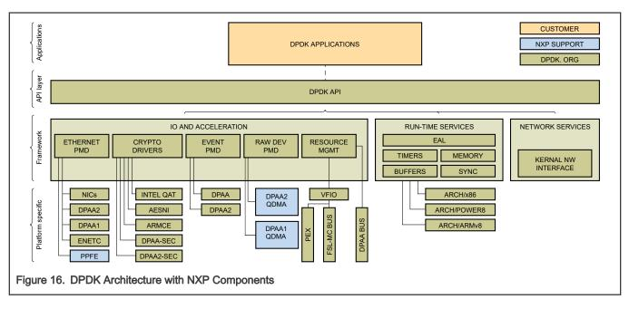
The NXP Data Path Acceleration Architecture comprises of a set of hardware components, which are integrated via a hardware queue manager and use a common hardware buffer manager. Software accesses the DPAA via hardware components called *"Software Portals"*. These directly provide queue and buffer manager operations, such as enqueues, dequeues, buffer allocations, and buffer releases and indirectly provide access to all of the other DPAA hardware components via the queue manager.
