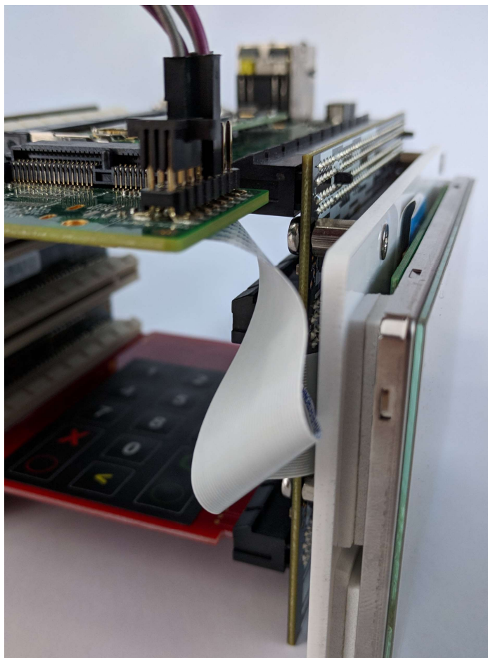
Figure 14. TWR-LCD ribbon connected to TWR-LPOS-RDR #2
