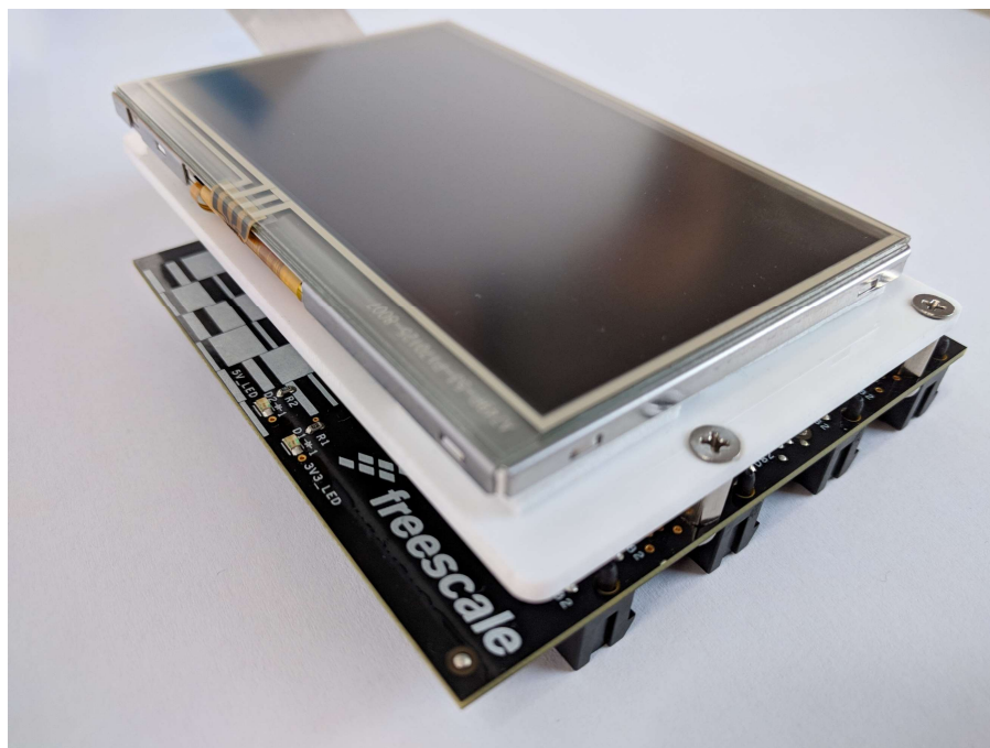
Figure 9. TWR-LCD connected on TWR-Elev Secondary
