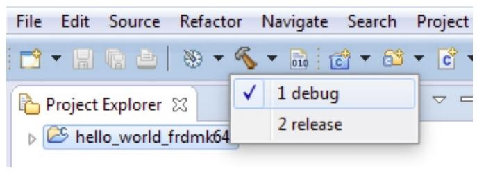
Figure 22. Selection of the build target in KDS IDE
