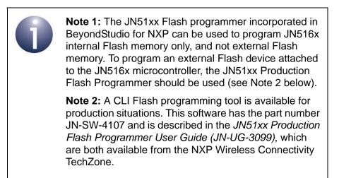
The integrated Flash programming tool also offers the facility to erase or program the JN516x EEPROM and to program a customer IEEE/MAC address into the target device. These items can be programmed at the same time as programming Flash memory or without programming Flash memory.
