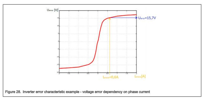
The inverter error characteristic is assigned to the GMCLIB\_DTCompLut1D algorithm as the LUT, which simply adds the error-voltage vector to the input-voltage vector. The data for the LUT should be measured from a real inverter for the best compensation result. The target of the measurement is the voltage-error-to-phase-current dependency, as shown in Figure 29.
