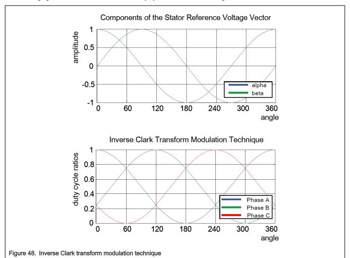
For an accurate calculation of the duty-cycle ratios and the direct- $\alpha$  and quadrature- $\beta$  components of the stator reference voltage vector, the duty cycle cannot be higher than one (100 %); in other words, the assumption
