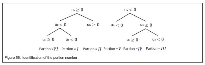
Finally, the corresponding duty cycle is selected according to the portion from the column of the following table.
