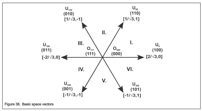
Referring to this principle, the objective of the standard space vector modulation is an approximation of the reference stator voltage vector U<sub>S</sub>, with an appropriate combination of the switching patterns, composed of basic space vectors. The graphical explanation of this objective is shown in Figure 3 and Figure 4.
