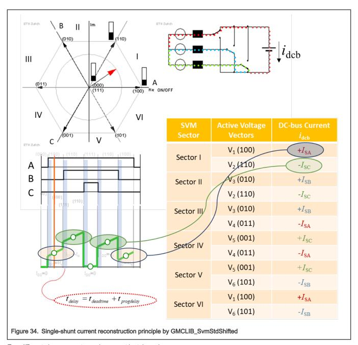
Two different phase-current samples cannot be taken when:
