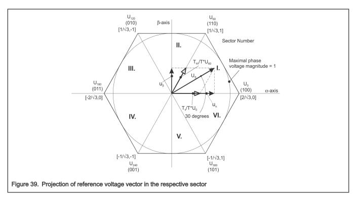
The stator reference voltage vector  $U_S$  is phase-advanced by 30° from the direct- $\alpha$ , and thus can be generated with an appropriate combination of the adjacent basic switching states  $U_0$  and  $U_{60}$ . These figures also indicate the resultant direct- $\alpha$  and quadrature- $\beta$  components for space vectors  $U_0$  and  $U_{60}$ .
