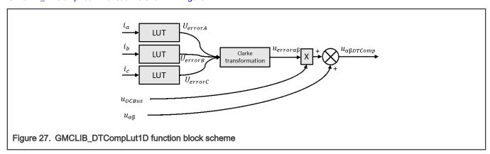
Adding the GMCLIB\_DTCompLut1D function into your application has the following essentials. Each inverter introduces the total error voltage, which is caused by the dead-time and current-clamping effects and the transistor voltage drop. The actual inverter output voltage is lower than the required voltage. The total error voltage depends on the actual phase current. The example of the inverter error characteristic is shown in Figure 28.
