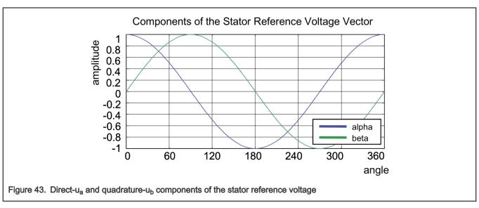
$\label{eq:gmclb_symStd_lmg7} GMCLIB\_SvmStd\_Img7 \ depicts \ the \ direct-u_{\alpha} \ and \ quadrature-u_{\beta} \ components \ of \ the \ stator \ reference \ voltage \ vector \ U_S, \ which \ were \ calculated \ using \ equations \ u_{\alpha} = \cos \vartheta \ and \ u_{\beta} = \sin \vartheta, \ respectively.$
