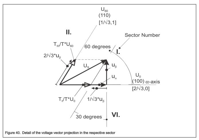
In this case, the reference stator voltage vector  $U_S$  is located in sector I, and can be generated using the appropriate duty-cycle ratios of the basic switching states  $U_0$  and  $U_{60}$ . The principal equations concerning this vector location are as follows:
