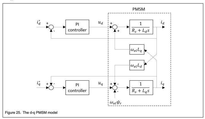
To eliminate the nonlinearity, the cross-coupling voltage is calculated using the GMCLIB\_DecouplingPMSM algorithm, and feedforwarded to the d and q voltages. The decoupling algorithm is calculated using the following equations:
