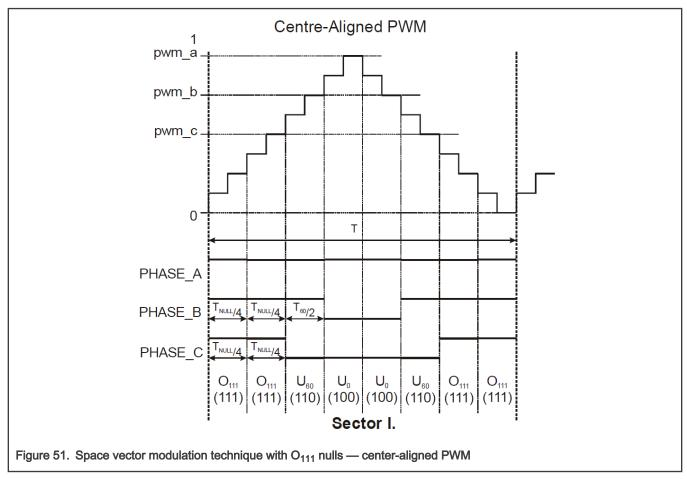
Figure GMCLIB\_SvmU7n\_Img1 shows calculated waveforms of the duty-cycle ratios using Space Vector Modulation with O<sub>111</sub> nulls.
