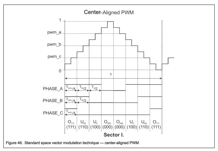
GMCLIB\_SvmStd\_Img11 shows the waveforms of the duty-cycle ratios, calculated using standard space vector modulation.
