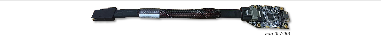
Figure 11. i.MX mini SAS cable with LVDS-to-HDMI adapter
