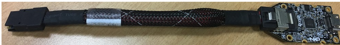
Figure 2. i.MX mini SAS cable with LVDS-to-HDMI adapter
