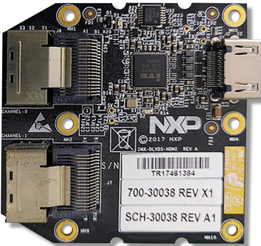
Figure 18. i.MX dual-channel LVDS-to-HDMI adapter
