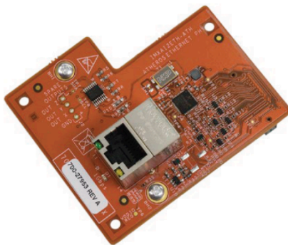
Figure 99. Atheros Ethernet add on card (IMXAI2ETH-ATH)
