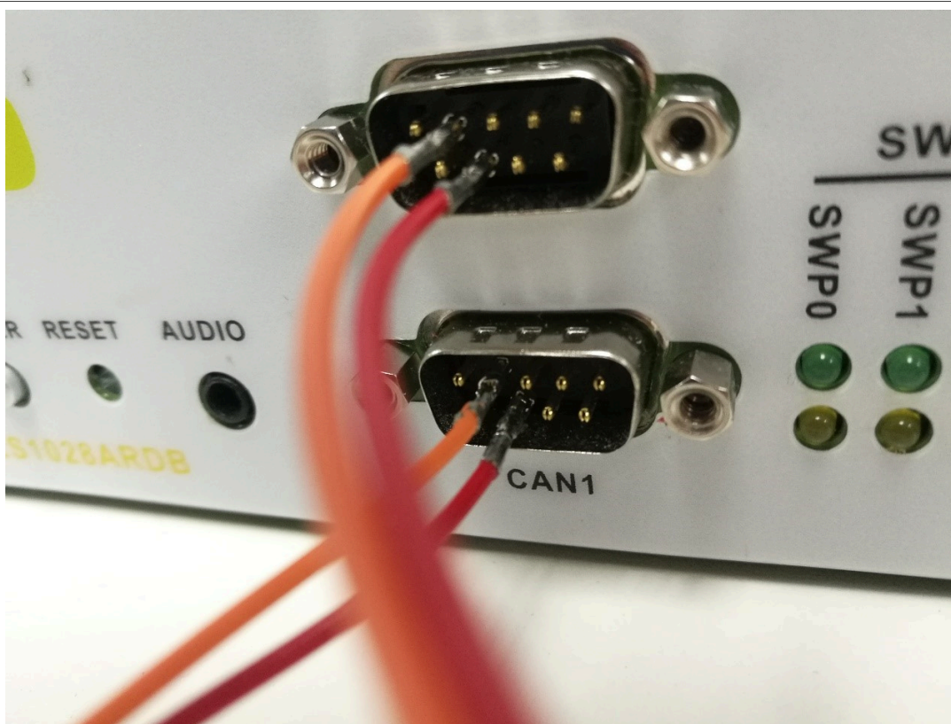
Figure 146. Physical connection for CAN using LS1028ARDB
