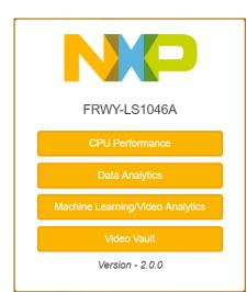
**CPU Performance Benchmarking** – Select CoreMark or Dhrystone to demonstrate the best-in-class CoreMarks/mW and DMIPS performance benchmarks of the LS1046A.
