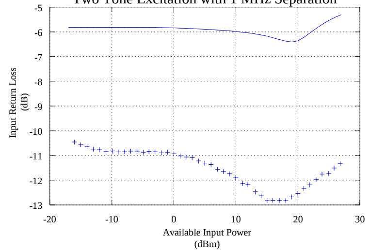
Input Return Loss vs. Available Input Power Two Tone Excitation with 1 MHz Separation
