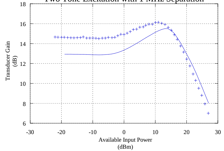
Transducer Gain vs. Available Input Power Two Tone Excitation with 1 MHz Separation
