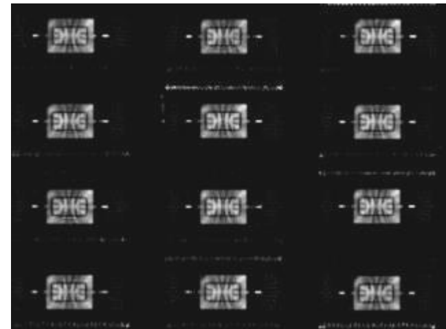
Scanning acoustic microscopy shows no delamination of die attach after 2000 cycles TC -50°C / +150°C
