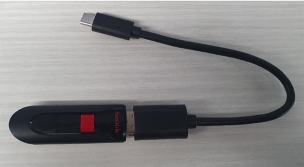
Figure 17. USB-C to USB adapter connections
