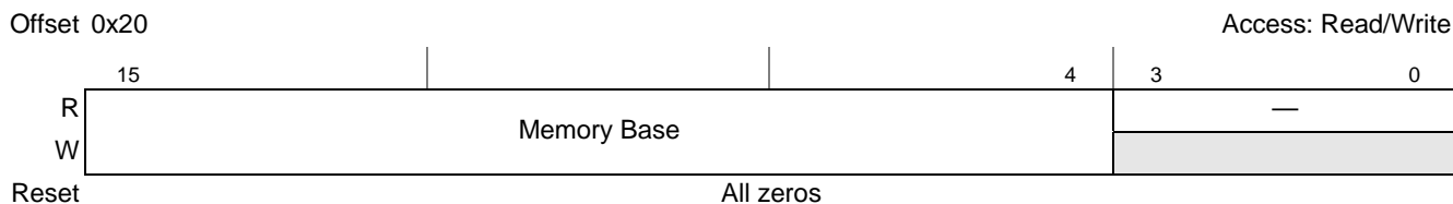
Figure 17-77. PCI Express Memory Base Register
