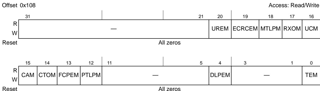
**Figure 17-115. PCI Express Uncorrectable Error Mask Register**
