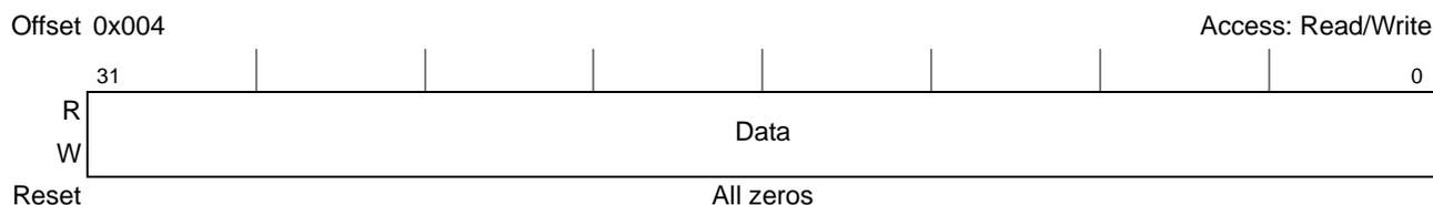
**Figure 17-13. PCI Express Configuration Data Register (PEX\_CONFIG\_DATA)**
