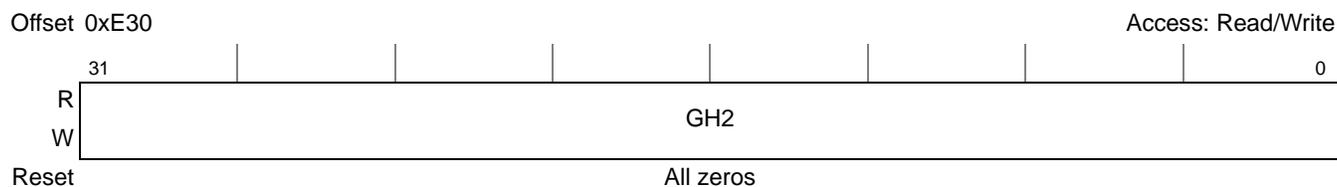
**Figure 17-44.** PCI Express Error Capture Register 2 (PEX\_ERR\_CAP\_R2)
