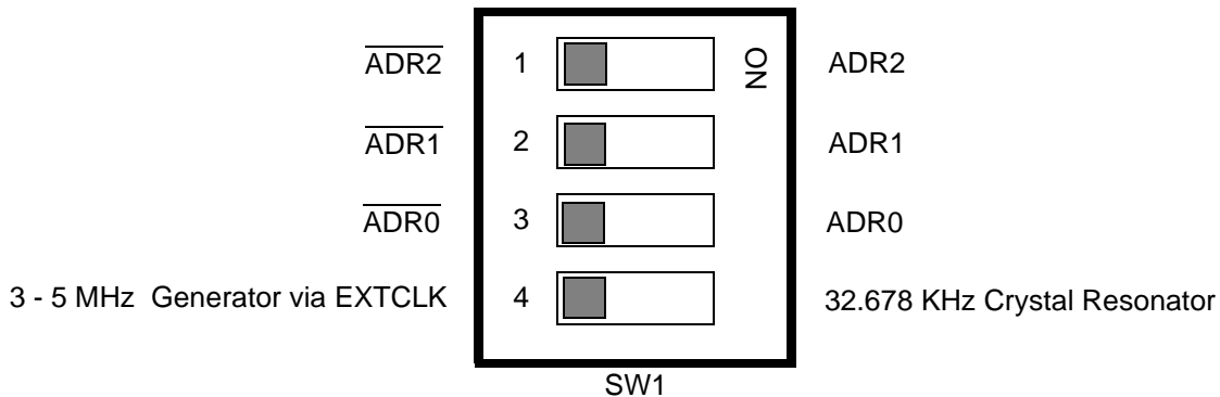
FIGURE 1-4 Configuration Dip-Switch - SW1
