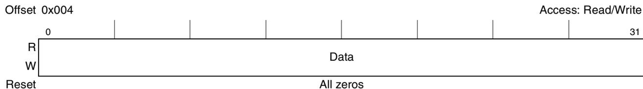
**Figure 17-3. PCI Express Configuration Data Register (PEX\_CONFIG\_DATA)**
