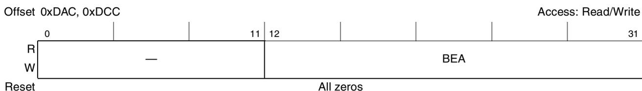
**Figure 16-13. PCI Inbound Window Base Extended Address Registers (PIWBEAR<sub>n</sub>)**
