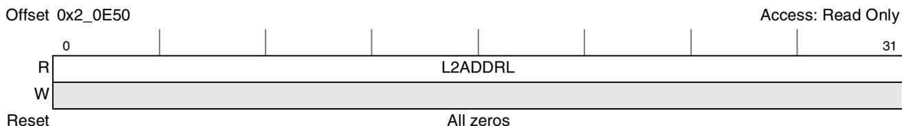
**Figure 6-23. L2 Error Address Capture Register (L2ERRADDRL)**
