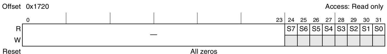
**Figure 9-32. Shared Message Signaled Interrupt Status Register (MSISR)**
