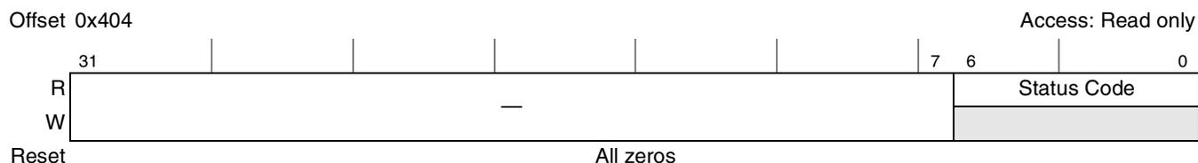
**Figure 17-114. PCI Express LTSSM State Status Register (PEX\_LTSSM\_STAT)**
