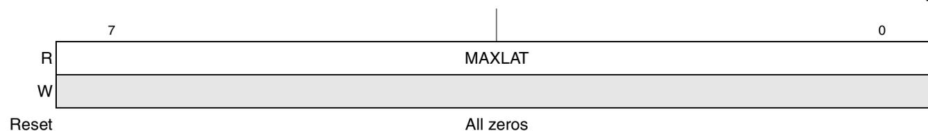
Figure 16-45. PCI Bus Maximum Latency Register (MAX\_LAT)
