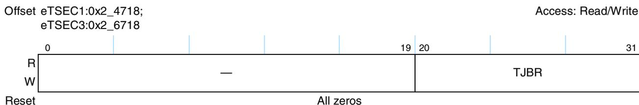
**Figure 14-92. Transmit Jabber Frame Counter Register Definition**
