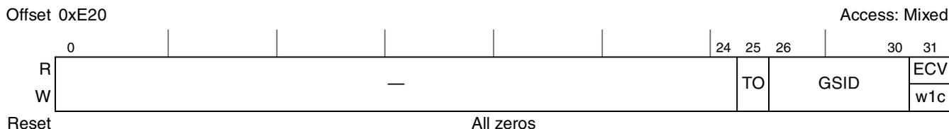
**Figure 17-27. PCI Express Error Capture Status Register (PEX\_ERR\_CAP\_STAT)**
