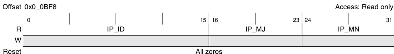
**Figure 2-2. Local Access IP Block Revision Register 1 (LAIPBRR1)**
