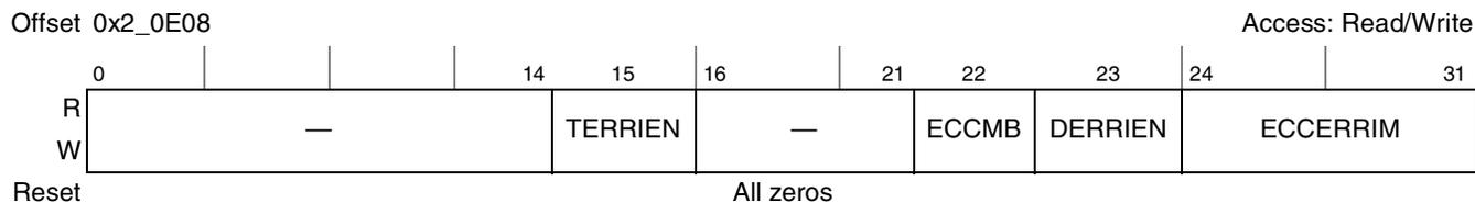
**Figure 6-15. L2 Error Injection Mask Control Register (L2ERRINJCTL)**
