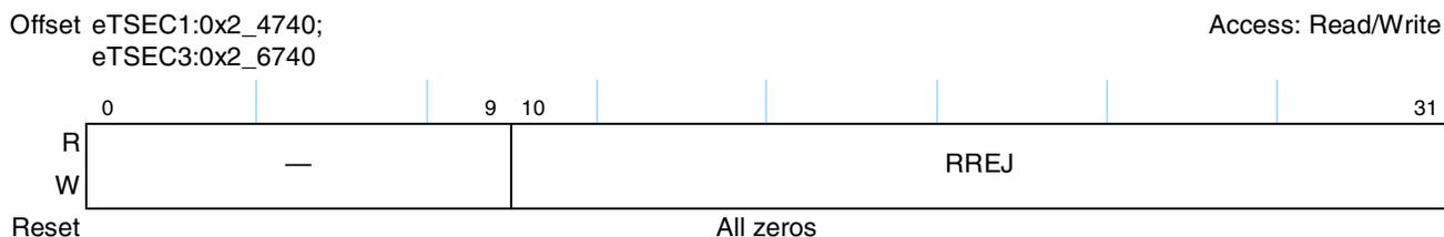
**Figure 14-102. Receive Filer Rejected Packet Counter Register Definition**
