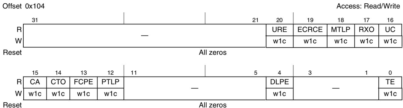
**Figure 17-103. PCI Express Uncorrectable Error Status Register**
