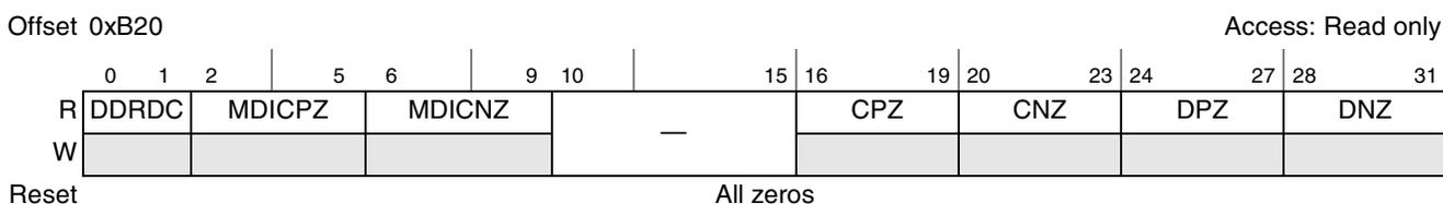
**Figure 8-26. DDR Debug Status Register 1 (DDRDSR\_1)**
