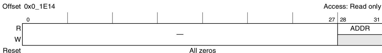
**Figure 7-10. ECM Error High Address Capture Register (EEHADR)**
