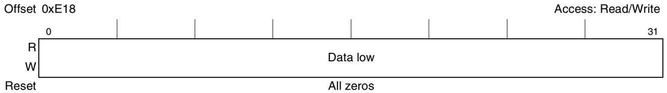
Figure 16-21. PCI Error Data Low Capture Register (ERR\_DL)
