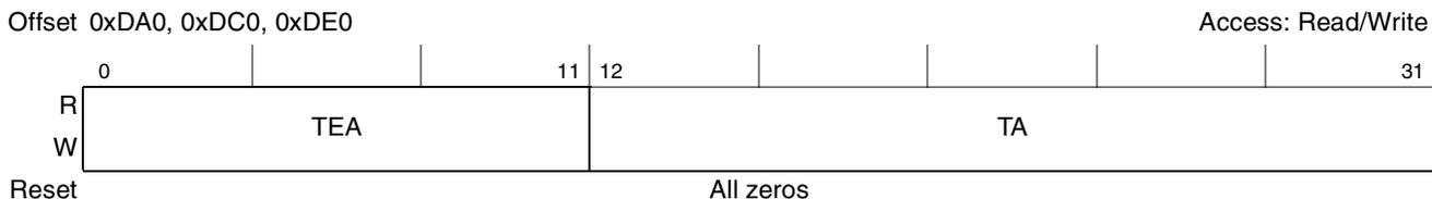
Figure 16-11. PCI Inbound Translation Address Registers (PITAR<sub>n</sub>)
