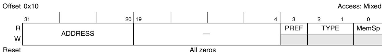
**Figure 17-59. PCI Express Base Address Register 0 (PEXCSRBAR)**
