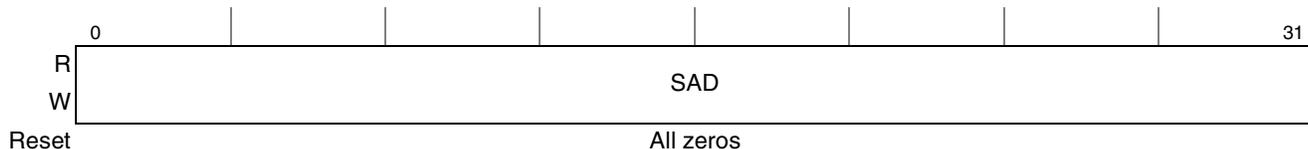
**Figure 15-10. Source Address Registers (SAR $n$ )**
