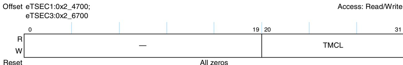
**Figure 14-87. Transmit Multiple Collision Packet Counter Register Definition**
