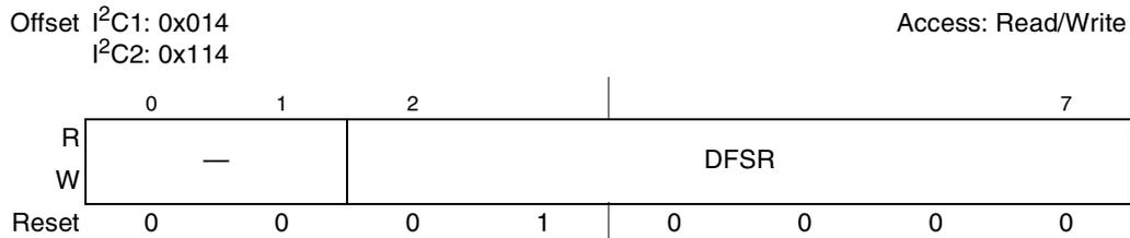
Figure 11-7. I<sup>2</sup>C Digital Filter Sampling Rate Register (I2CDFSRR)
