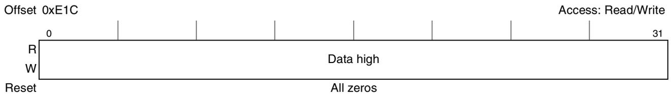
Figure 16-22. PCI Error Data High Capture Register (ERR\_DH)
