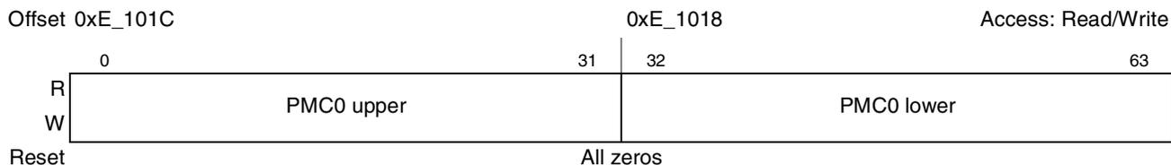
**Figure 24-7. Performance Monitor Counter Register 0 (PMC0)**
