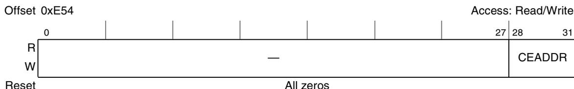
**Figure 8-43. Memory Error Extended Address Capture Register (CAPTURE\_EXT\_ADDRESS)**
