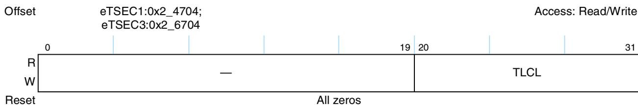
**Figure 14-88. Transmit Late Collision Packet Counter Register Definition**
