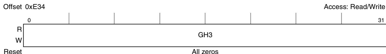
**Figure 17-35. PCI Express Error Capture Register 3 (PEX\_ERR\_CAP\_R3)
