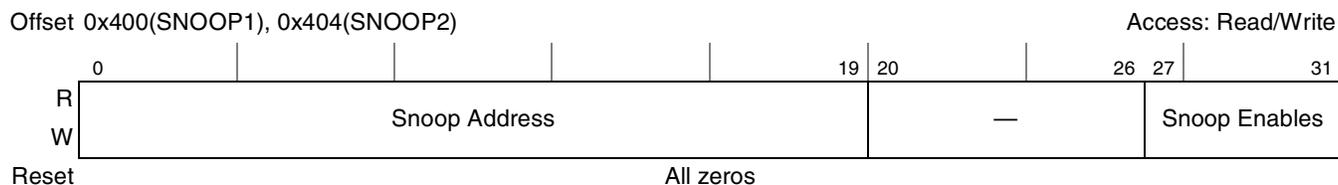
**Figure 21-29. Snoop 1 and Snoop 2 (SNOOP $n$ )**
