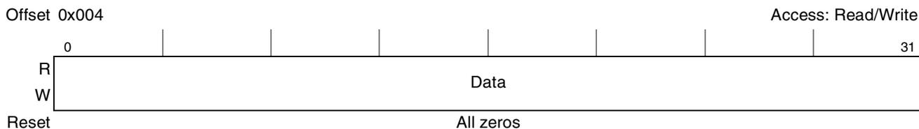
**Figure 16-4. PCI CFG\_DATA Register**
