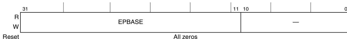
Figure 21-15. Endpoint List Address (ENDPOINTLISTADDR)
