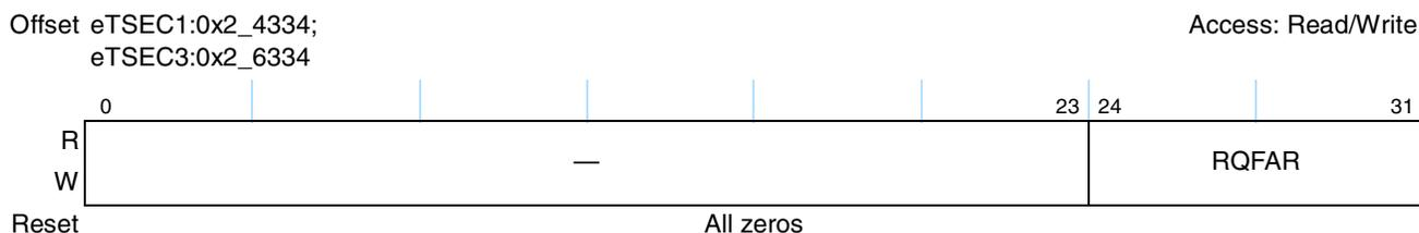
**Figure 14-29. Receive Queue Filer Table Address Register Definition**
