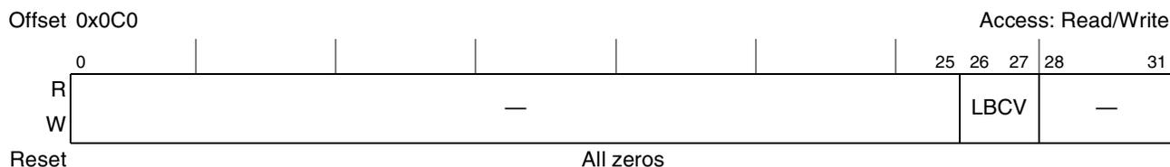
**Figure 23-23. LBC Voltage Select Control Register (LBCVSELCR)**
