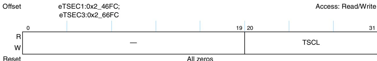
Figure 14-86. Transmit Single Collision Packet Counter Register Definition
