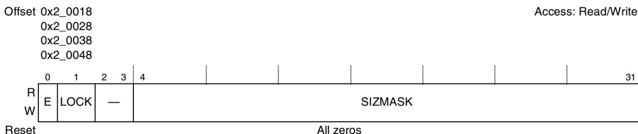
**Figure 6-10. Cache External Write Control Registers (L2CEWCR0–L2CEWCR3)**
