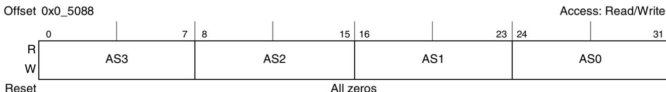
Figure 13-10. FCM Data Register in FCM Mode (MDR)
