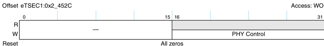
**Figure 14-47. MII Mgmt Control Register Definition**
