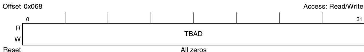
**Figure 25-16. Trace Buffer Access Data Register (TBADR)**
