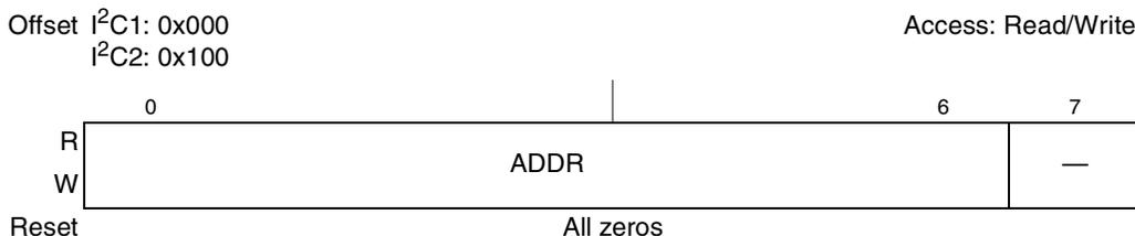
Figure 11-2. I<sup>2</sup>C Address Register (I2CADR)
