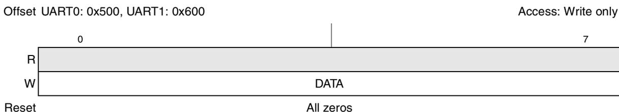
**Figure 12-3. Transmitter Holding Registers (UTHR<sub>n</sub>)**
