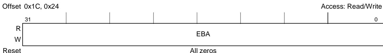
Figure 13-34. GPL Extended Base Address Registers 1–2
