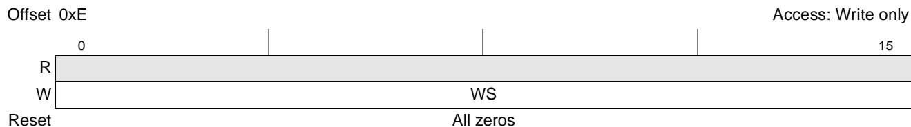
Figure 5-18. System Watchdog Service Register (SWSRR)
