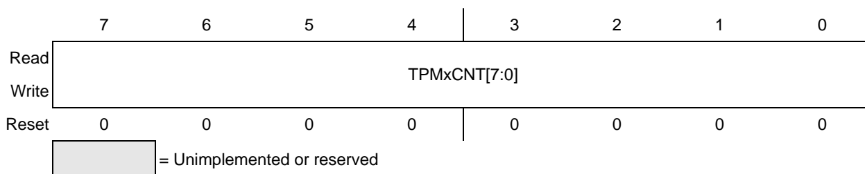
Figure 18-7. TPM Counter Register High (TPMxCNTH)
