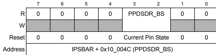
Figure 12-26. Port BS Pin Data/Set Data Register (PPDSDR_BS)
