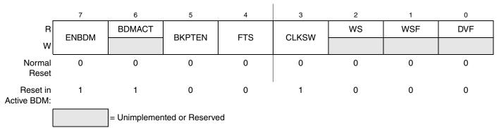
Figure 19-5. BDC Status and Control Register (BDCSCR)
