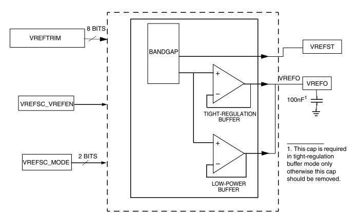
Figure 18-3. Voltage Reference Block Diagram
