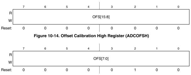
Figure 10-15. Offset Calibration Low Register (ADCOFSL)
