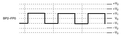
Figure 13-21. "e" Segment Voltage Waveform
