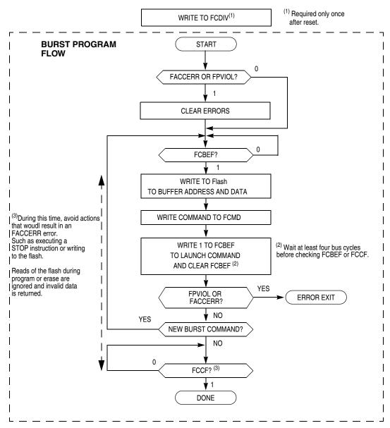
Figure 4-10. Flash Burst Program Flowchart
