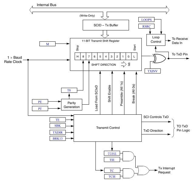
Figure 14-2. SCI Transmitter Block Diagram
