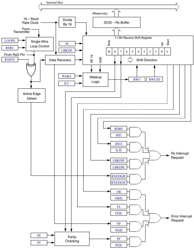
Figure 14-3. SCI Receiver Block Diagram
