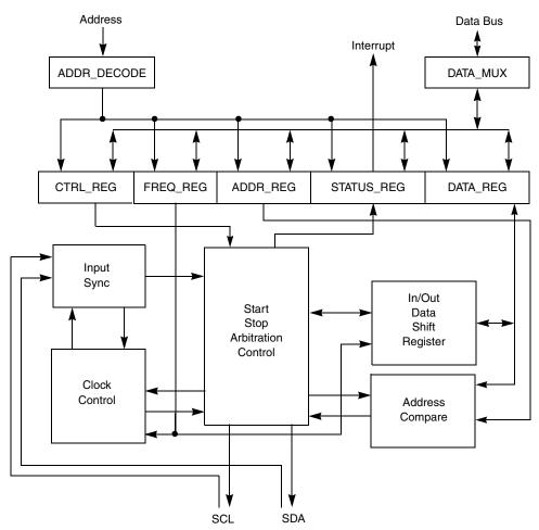
Figure 12-2. IIC Functional Block Diagram
