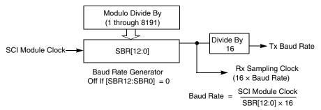
Figure 14-12. SCI Baud Rate Generation
