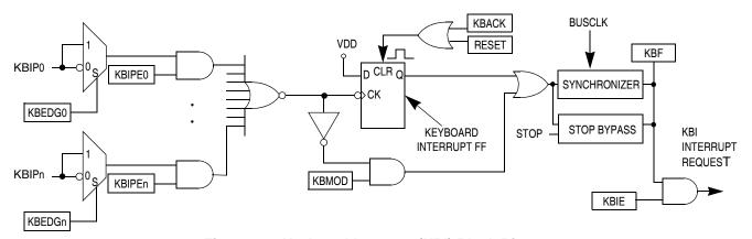
Figure 7-2. Keyboard Interrupt (KBI) Block Diagram
