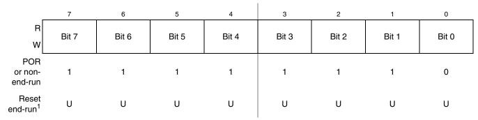
Figure 20-3. Debug Comparator A Low Register (DBGCAL)
