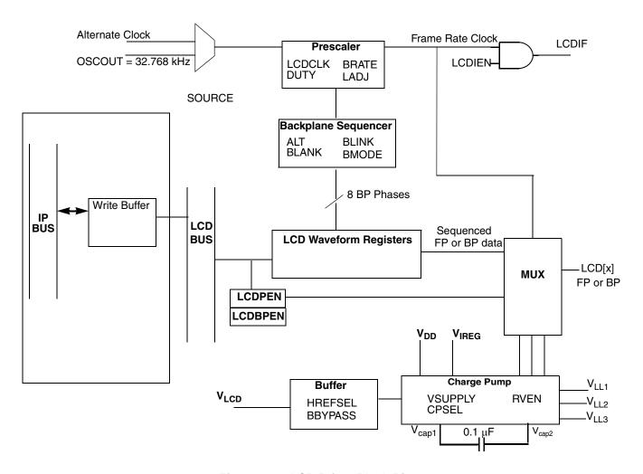
Figure 13-2. LCD Driver Block Diagram
