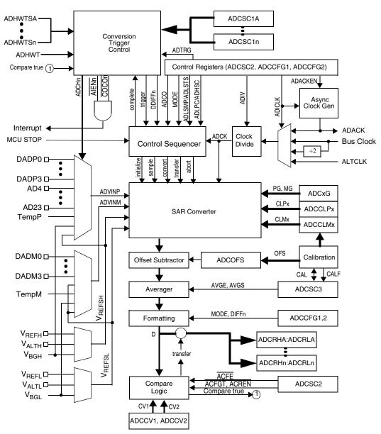
Figure 10-2. ADC Block Diagram
