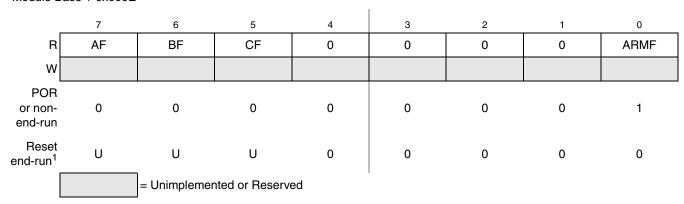
Figure 20-16. Debug Status Register (DBGS)
