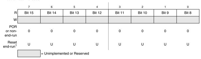
Figure 20-8. Debug FIFO High Register (DBGFH)
