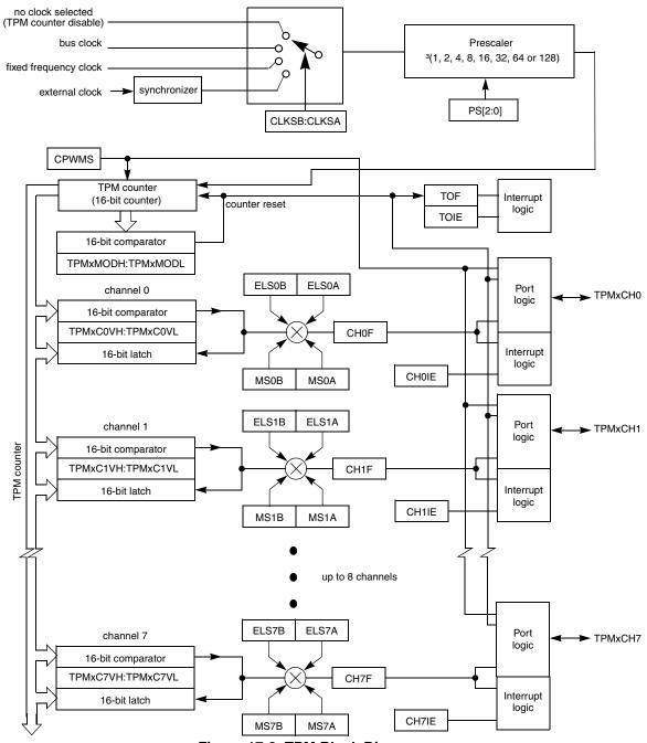
Figure 17-2. TPM Block Diagram
