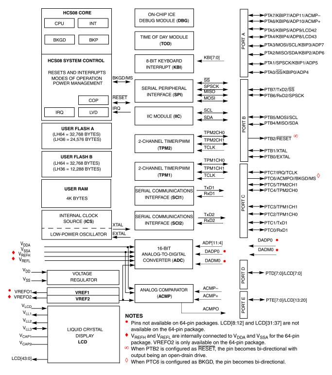
Figure 1-1. MC9S08LH64 Series Block Diagram
