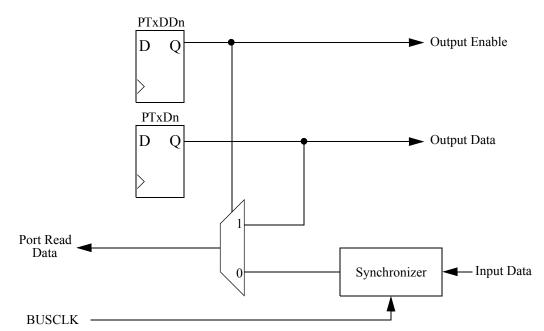
Figure 6-1. Parallel I/O Block Diagram
