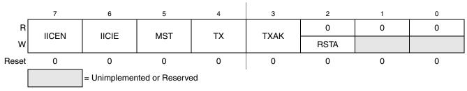
Figure 12-5. IIC Control Register (IICC1)
