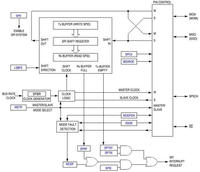
Figure 15-3. SPI Module Block Diagram
