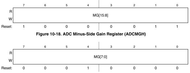
Figure 10-19. ADC Minus-Side Gain Register (ADCMGL)
