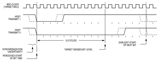
Figure 19-2. BDC Host-to-Target Serial Bit Timing
