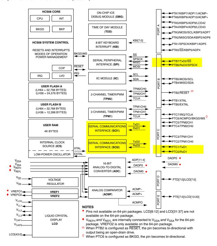
Figure 14-1. MC9S08LH64 Series Block Diagram Highlighting SCI Blocks and Pins
