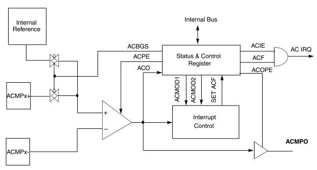
Figure 9-2. Analog Comparator Module Block Diagram
