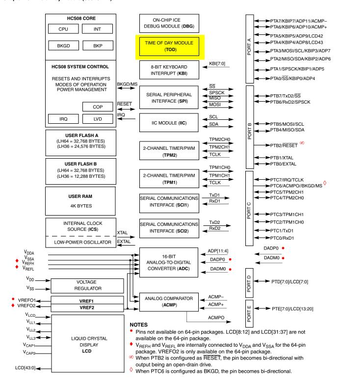
Figure 16-1. MC9S08LH64 Block Diagram Highlighting TOD Block and Pins
