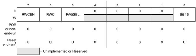
Figure 20-12. Debug Comparator C Extension Register (DBGCCX)
