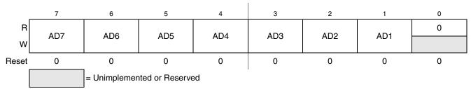
Figure 12-3. IIC Address Register (IICA)
