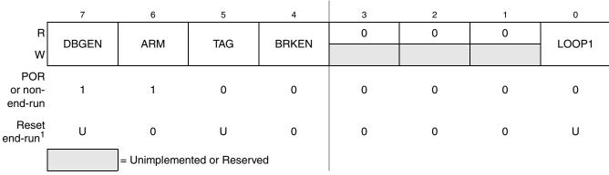
Figure 20-14. Debug Control Register (DBGC)
