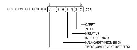
Figure 8-2. Condition Code Register
