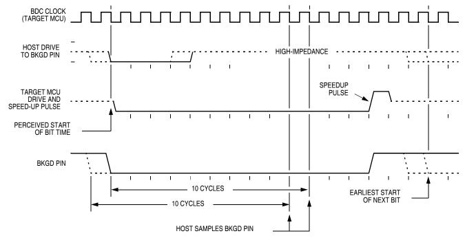
Figure 19-4. BDM Target-to-Host Serial Bit Timing (Logic 0)
