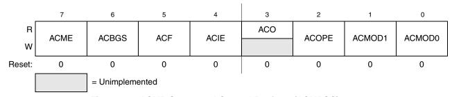
Figure 9-3. ACMP Status and Control Register (ACMPSC)
