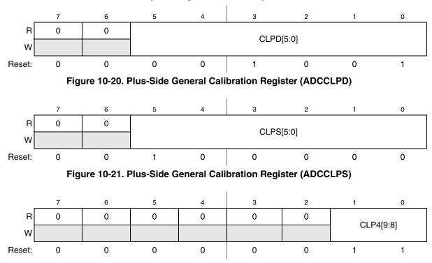
Figure 10-22. Plus-Side General Calibration Register (ADCCLP4H)
