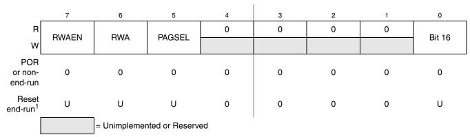
Figure 20-10. Debug Comparator A Extension Register (DBGCAX)
