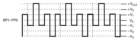
Figure 13-20. "f" Segment Voltage Waveform
