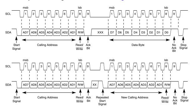
Figure 12-9. IIC Bus Transmission Signals
