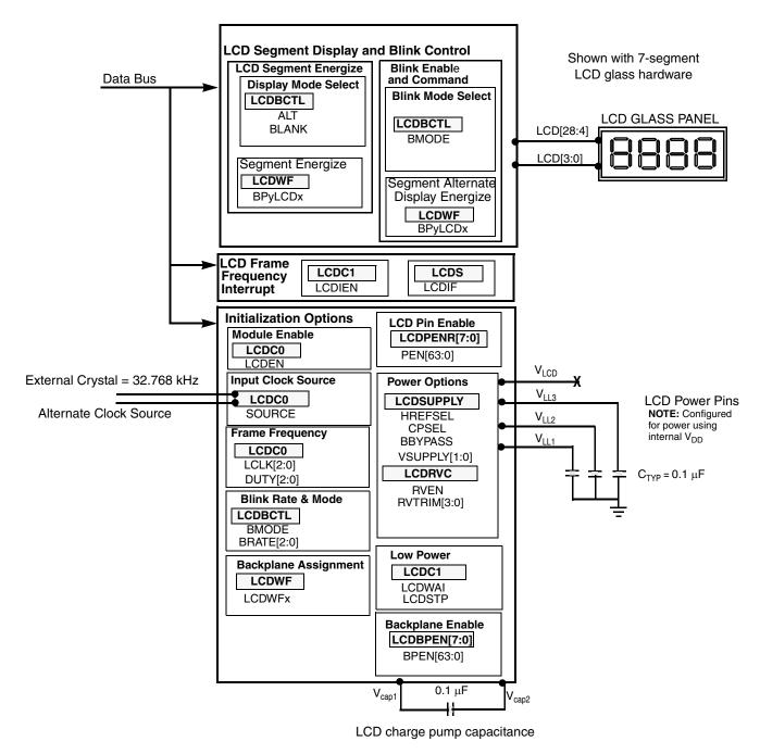
Figure 13-17. LCD Programmer's Model Diagram
