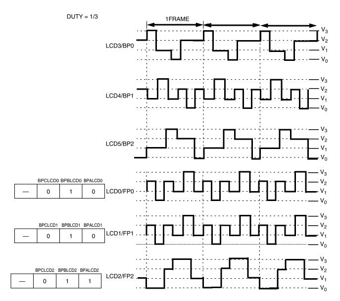
Figure 13-19. LCD Waveforms
