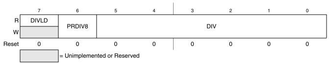
Figure 4-12. Flash Clock Divider Register (FCDIV)
