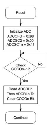
Figure 10-42. Initialization Flowchart for Example
