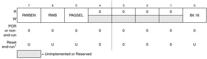
Figure 20-11. Debug Comparator B Extension Register (DBGCBX)
