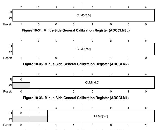
Figure 10-37. Minus-Side General Calibration Register (ADCCLM0)
