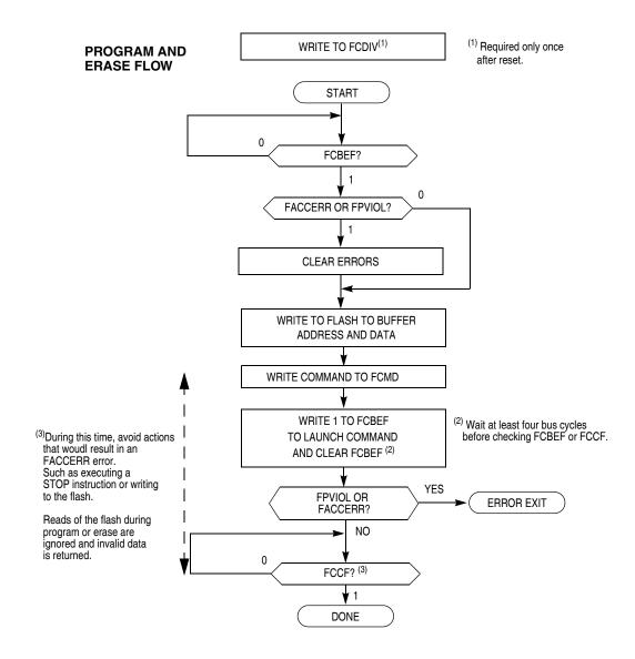
Figure 4-9. Flash Program and Erase Flowchart
