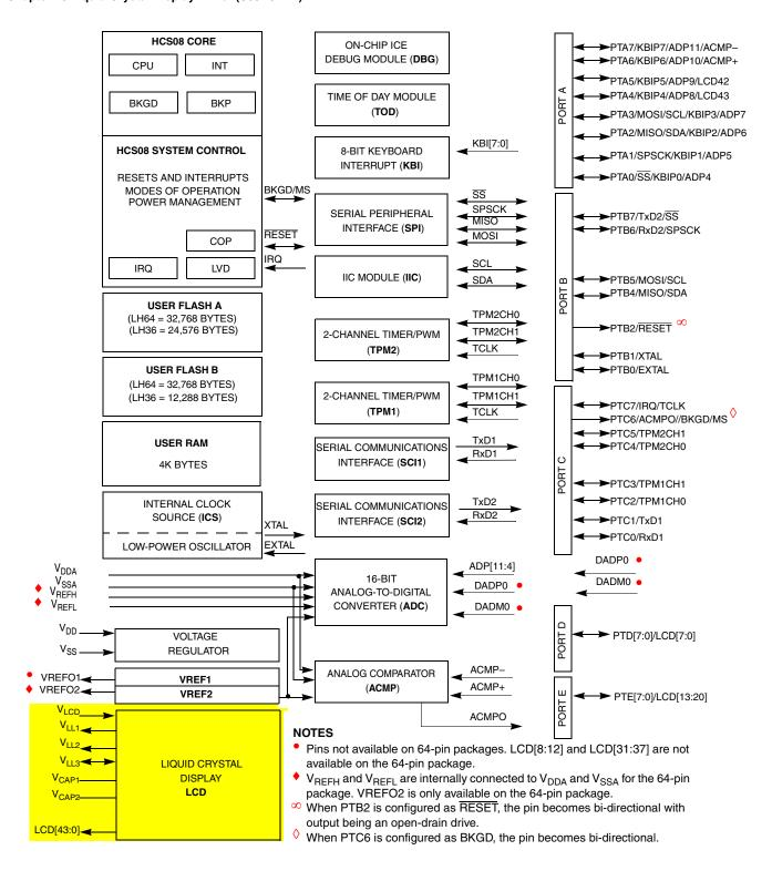
Figure 13-1. MC9S08LH64 Block Diagram Highlighting LCD Block and Pins
