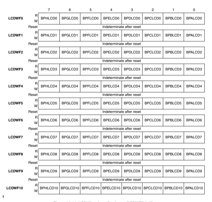
Figure 13-11. LCD Waveform Registers (LCDWF[63:0])
