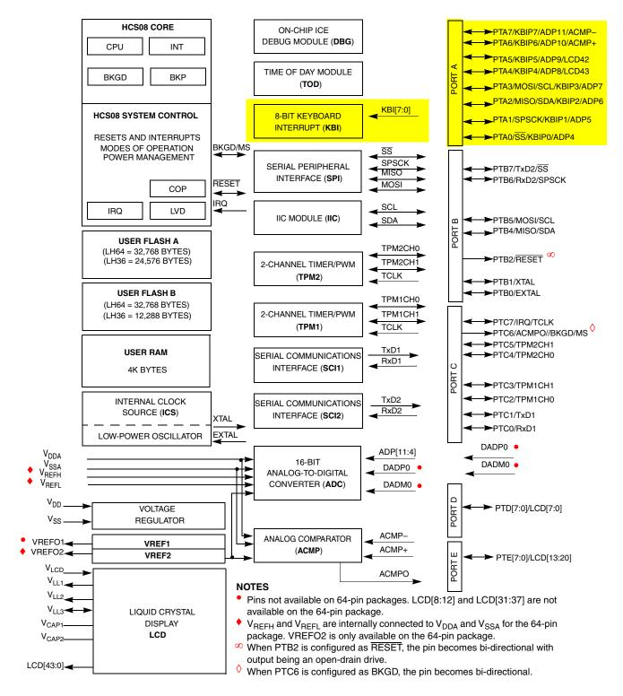
Figure 7-1. MC9S08LH64 Series Block Diagram Highlighting KBI Block and Pins
