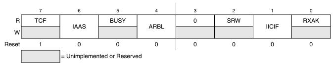
Figure 12-6. IIC Status Register (IICS)
