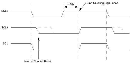
Figure 12-10. IIC Clock Synchronization
