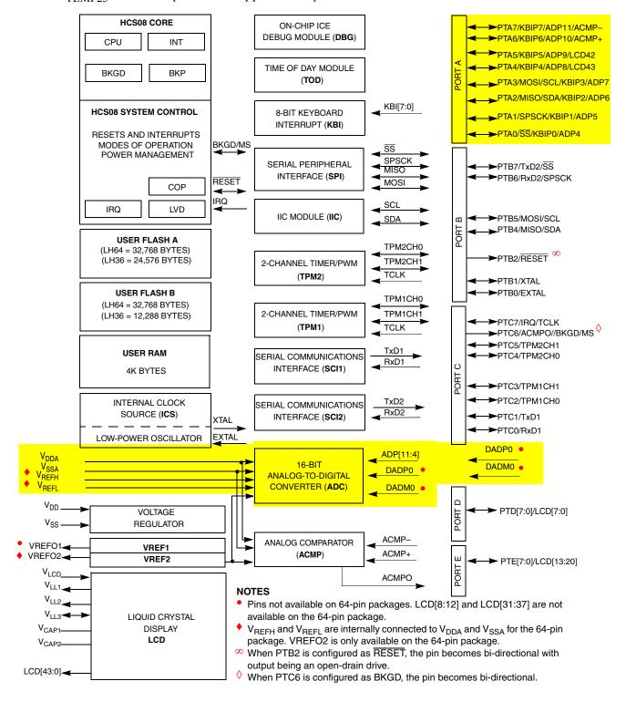
Figure 10-1. MC9S08LH64 Series Block Diagram Highlighting ADC Block and Pins
