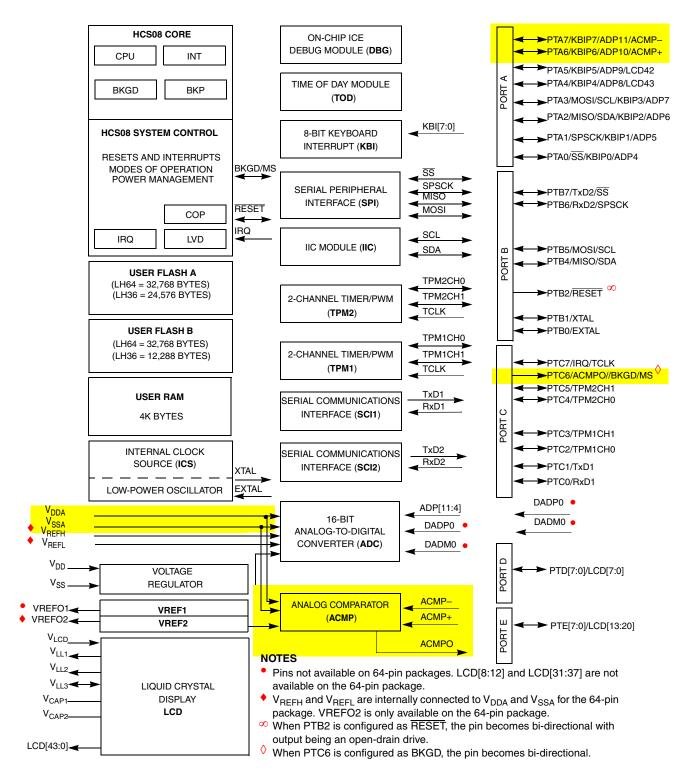
Figure 9-1. MC9S08LH64 Series Block Diagram Highlighting ACMP Block and Pins
