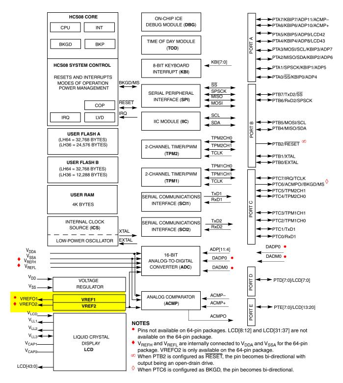
Figure 18-1. MC9S08LH64 Series Block Diagram Highlighting VREF Blocks and Pins
