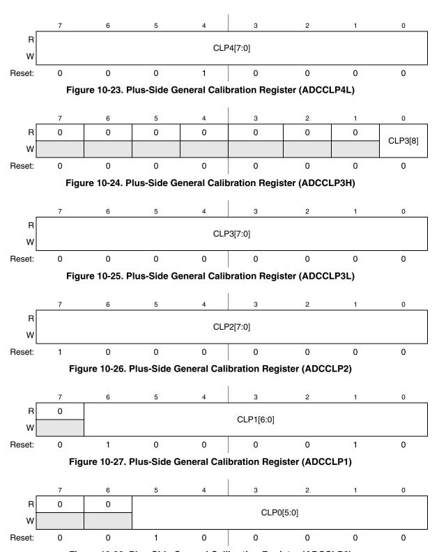
Figure 10-28. Plus-Side General Calibration Register (ADCCLP0)
