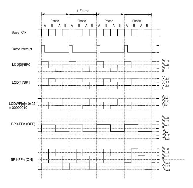
Figure 13-13. 1/2 Duty and 1/3 Bias (Low-Power Waveform)
