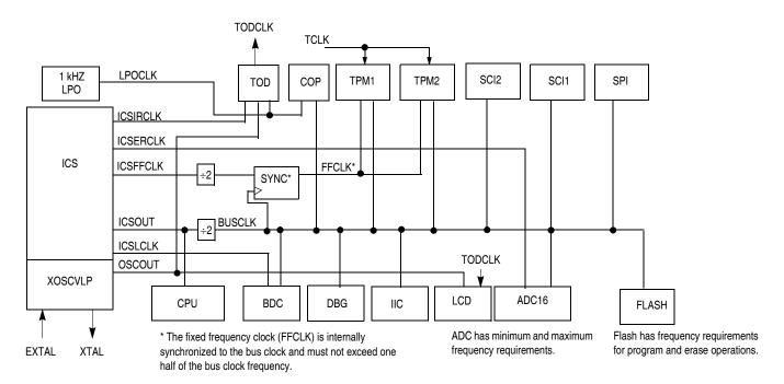
Figure 1-2. System Clock Distribution Diagram
