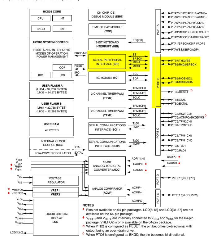
Figure 15-1. MC9S08LH64 Series Block Diagram Highlighting SPI Block and Pins
