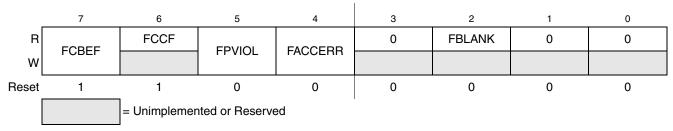
Figure 4-16. Flash Status Register (FSTAT)
