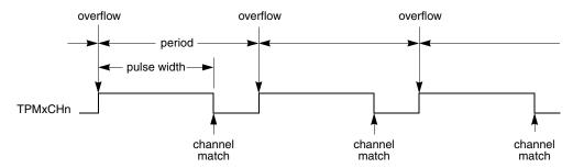
Figure 17-15. EPWM period and pulse width (ELSnA=0)
