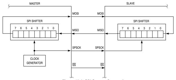
Figure 15-2. SPI System Connections
