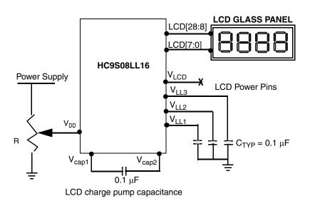
Figure 13-22. Power Connections for Contrast Control
