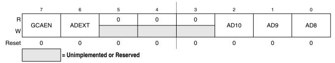
Figure 12-8. IIC Control Register (IICC2)
