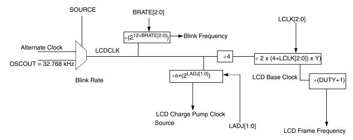
Figure 13-12. LCD Clock Tree
