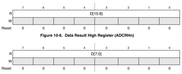
Figure 10-7. Data Result Low Register (ADCRLn)
