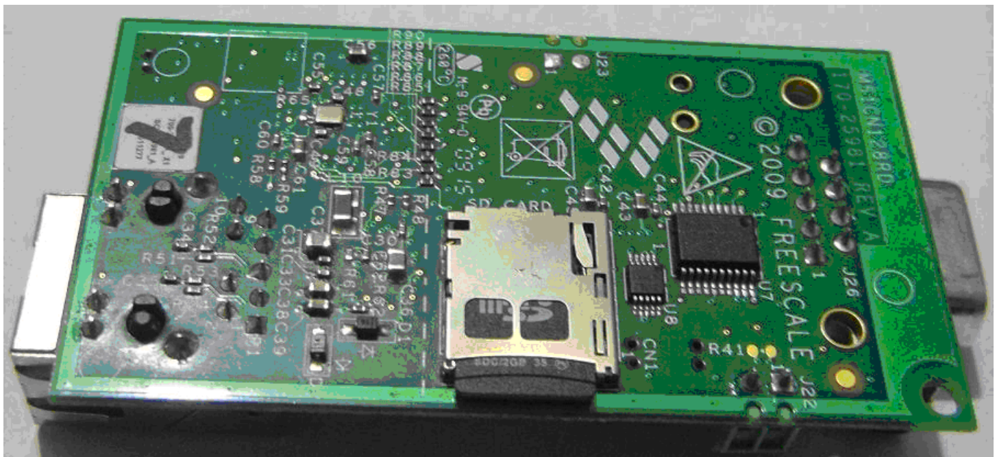
Figure 1-2. Bottom view of MCF51CN128 reference design hardware
