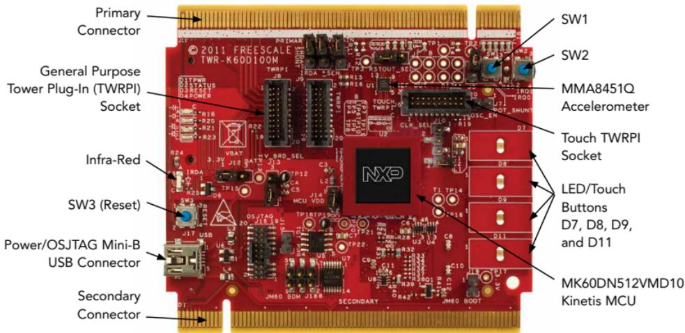
Figure 1: Front side of TWR-K60D100M module
