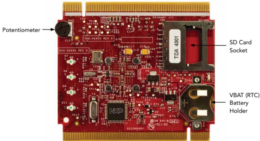
Figure 2: Back side of TWR-K6D100M module
