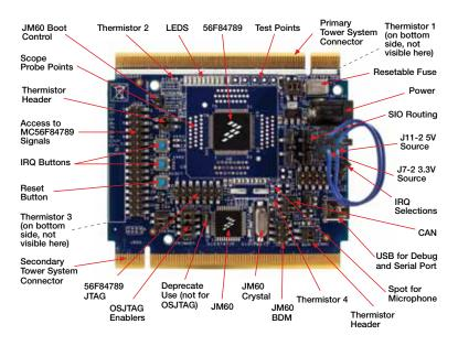
TWR-56F8400 is part of the Freescale Tower System portfolio, a modular development platform that enables rapid prototyping and tool re-use through reconfigurable hardware.
