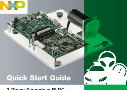
**3-Phase Sensorless BLDC Motor Control Development Kit**with Qorivva MPC5606B MCU
