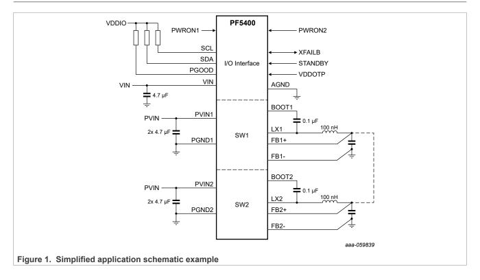
30 A dual phase high efficiency core supply regulator with AVP and watchdog
