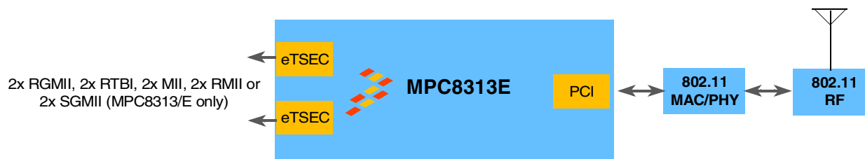
Figure 5. MPC8313E as a WLAN Access Point
