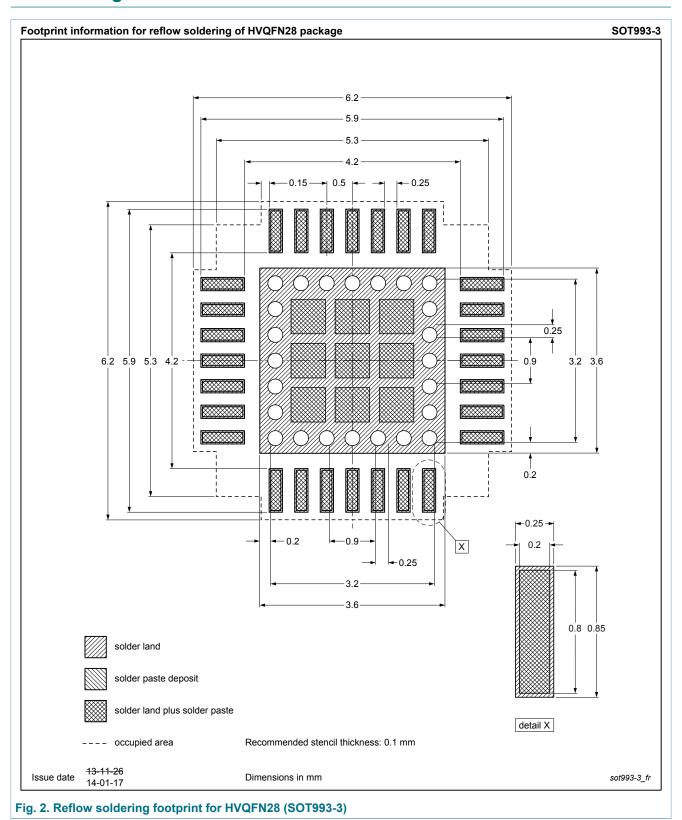
HVQFN28: plastic thermal enhanced very thin quad flat package; no leads; 28 terminals
