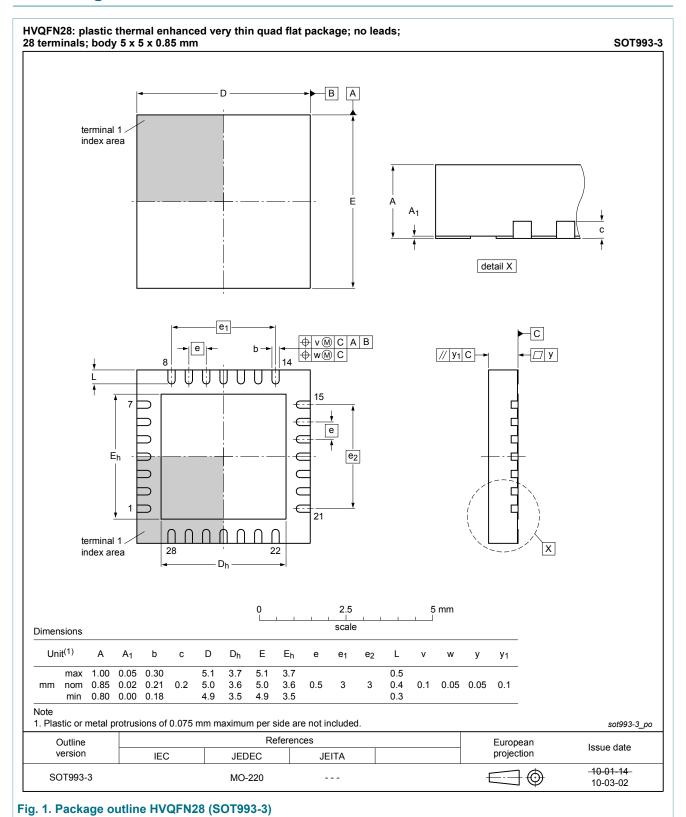
HVQFN28: plastic thermal enhanced very thin quad flat package; no leads; 28 terminals
