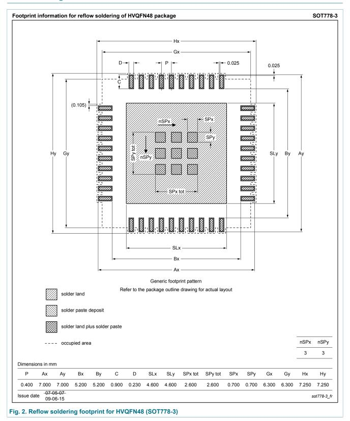
plastic thermal enhanced very thin quad flat package; no leads; 48 terminals; body 6 x 6 x 0.85 mm
