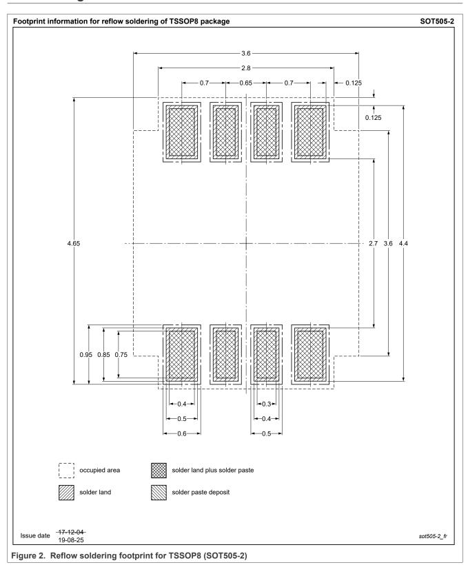
TSSOP8, thin shrink small outline package; 8 leads; 0.65 mm pitch; 3 mm x 3 mm x 1.1 mm body
