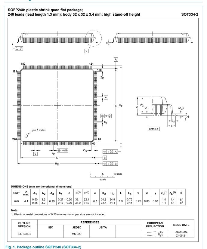
plastic shrink quad flat package; 240 leads (lead length 1.3 mm); body 32 x 32 x 3.4 mm; high stand-off height
