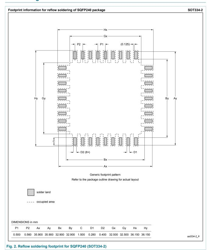
plastic shrink quad flat package; 240 leads (lead length 1.3 mm); body 32 x 32 x 3.4 mm; high stand-off height
