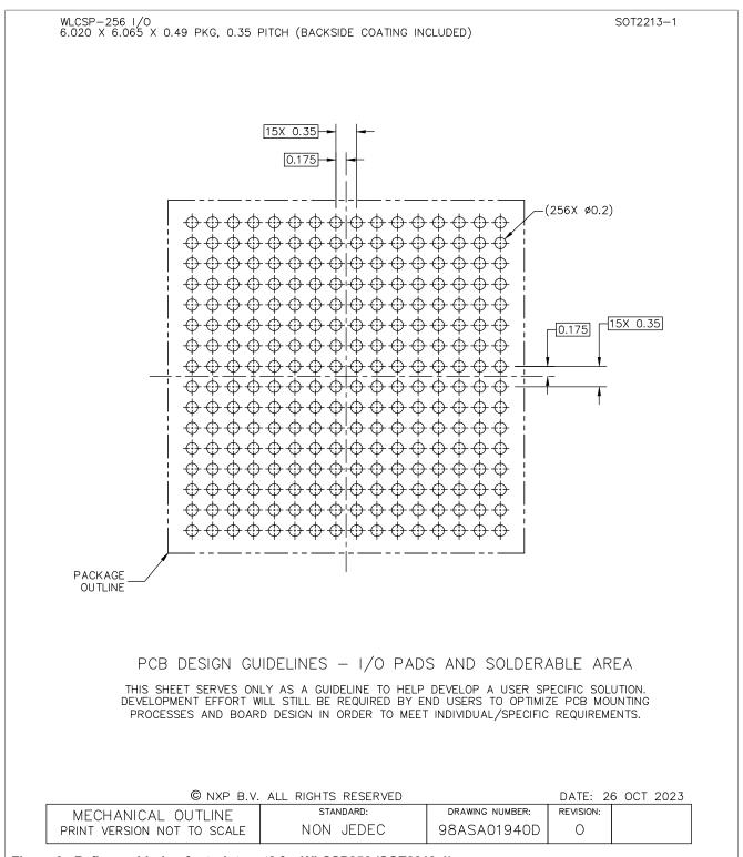
Figure 3. Reflow soldering footprint part2 for WLCSP256 (SOT2213-1)
