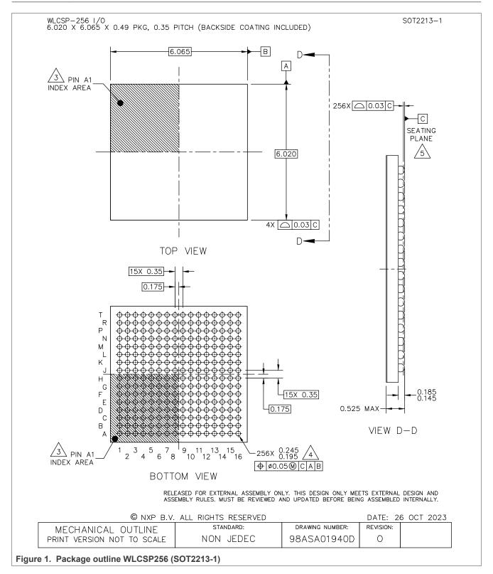
WLCSP256, wafer level chip-size package, 256 terminals, 0.35 mm pitch, 6.02 mm x 6.065 mm x 0.49 mm body
