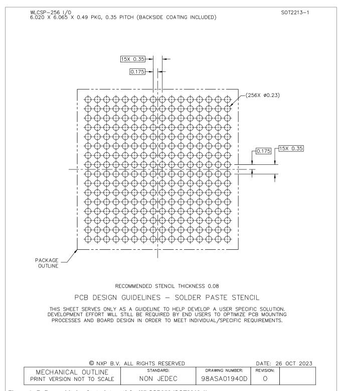
Figure 4. Reflow soldering footprint part3 for WLCSP256 (SOT2213-1)
