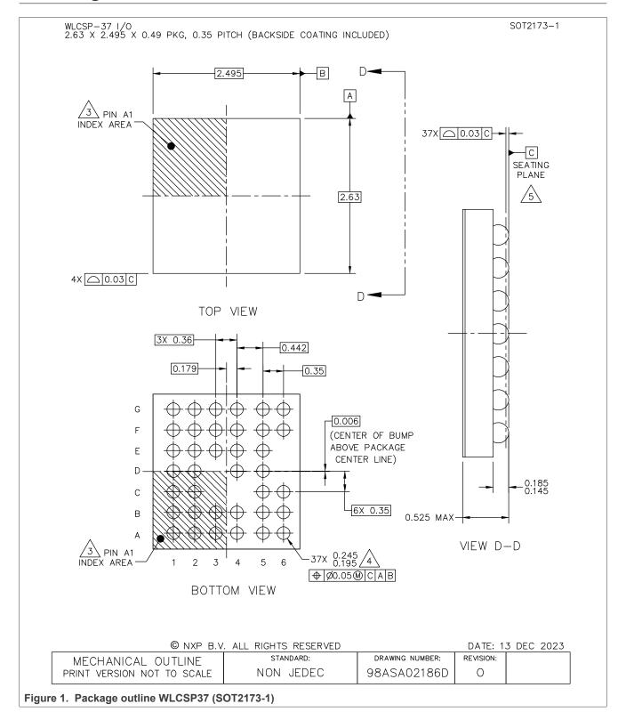
WLCSP37, wafer level chip-size package; 37 terminals; 0.35 mm pitch; 2.63 mm x 2.495 mm x 0.49 mm body
