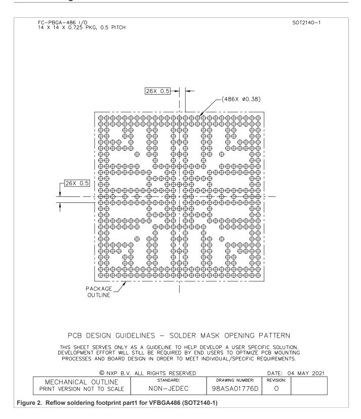
VFBGA486, very thin fine-pitch ball grid array package, 486 terminals, 0.5 mm pitch, 14 mm x 14 mm x 0.725 mm body
