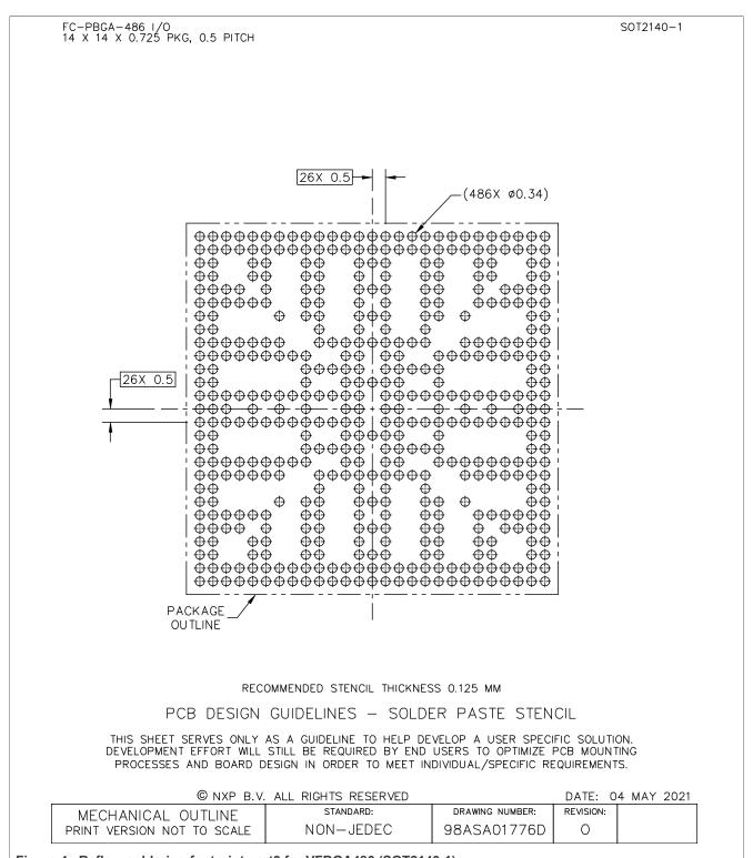
Figure 4. Reflow soldering footprint part3 for VFBGA486 (SOT2140-1)
