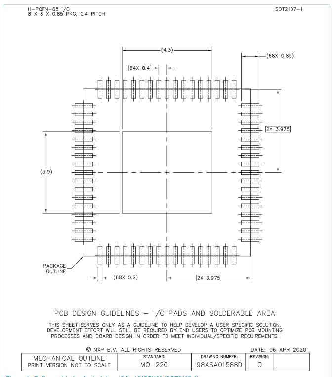
Figure 4. Reflow soldering footprint part2 for HVQFN68 (SOT2107-1)
