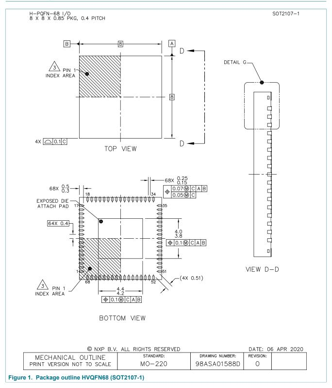
HVQFN68, thermal enhanced very thin quad flat package, no leads, 68 terminals, 0.4 mm pitch, 8 mm x 8 mm x 0.85 mm body
