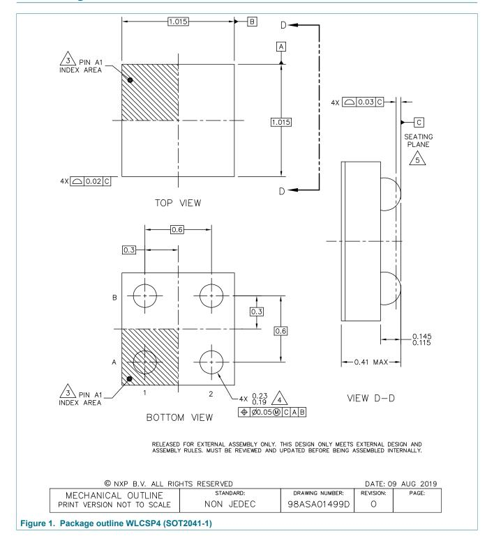
WLCSP4, wafer level chip scale package, 4 terminals; 0.6 mm pitch; 1.015 mm x 1.015 mm x 0.38 mm body (backside coating included)
